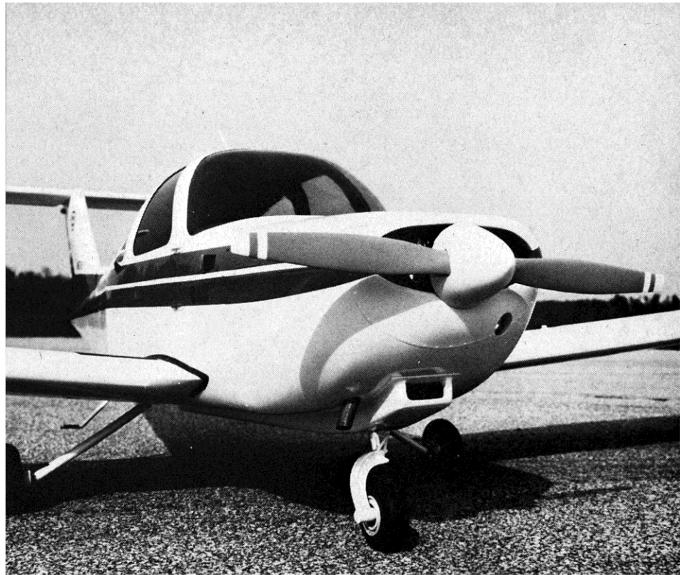
The cowl can be either carved out of balsa, or formed with the foam/wax lay-up technique. The lines are very basic, and easy to duplicate.
