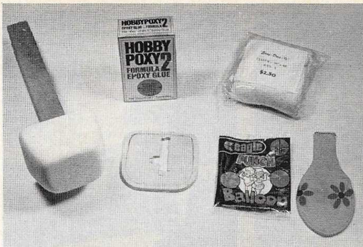
All the ingredients to make a Hobbypoxy Easy-Does-It type cowl. Note styrofoam mold at left mounted on a common 2x3. Former F-1A in center. Right: Balloon in place covering the complete mold. Remove it tomorrow.
