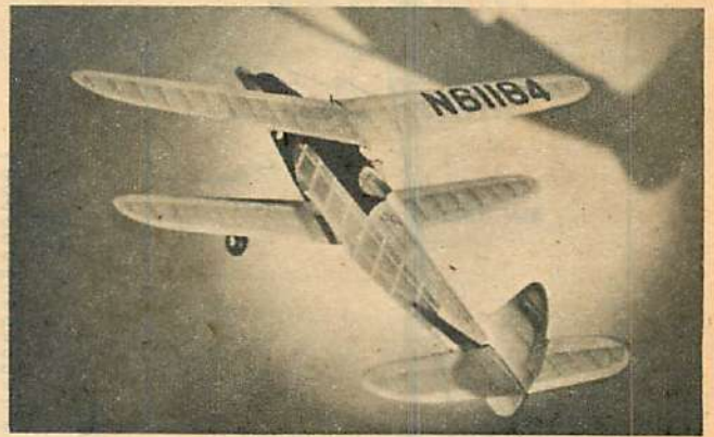
This beauty is powered by 18 strands of 1/4-inch flat T-56 rubber; to make building easy, full-size plans are available from Air Trails.
