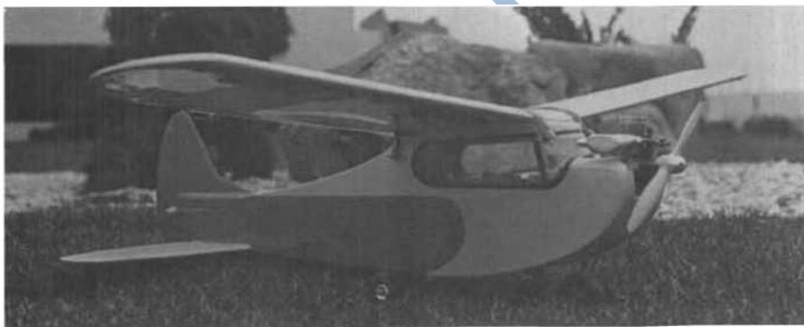
The Beam had the typical force set up of the day .. . high thrust line, low stab. DeBolt's "Live-wire Trainer" had similar set up .. . was equally popular. Good view into the cabin!
