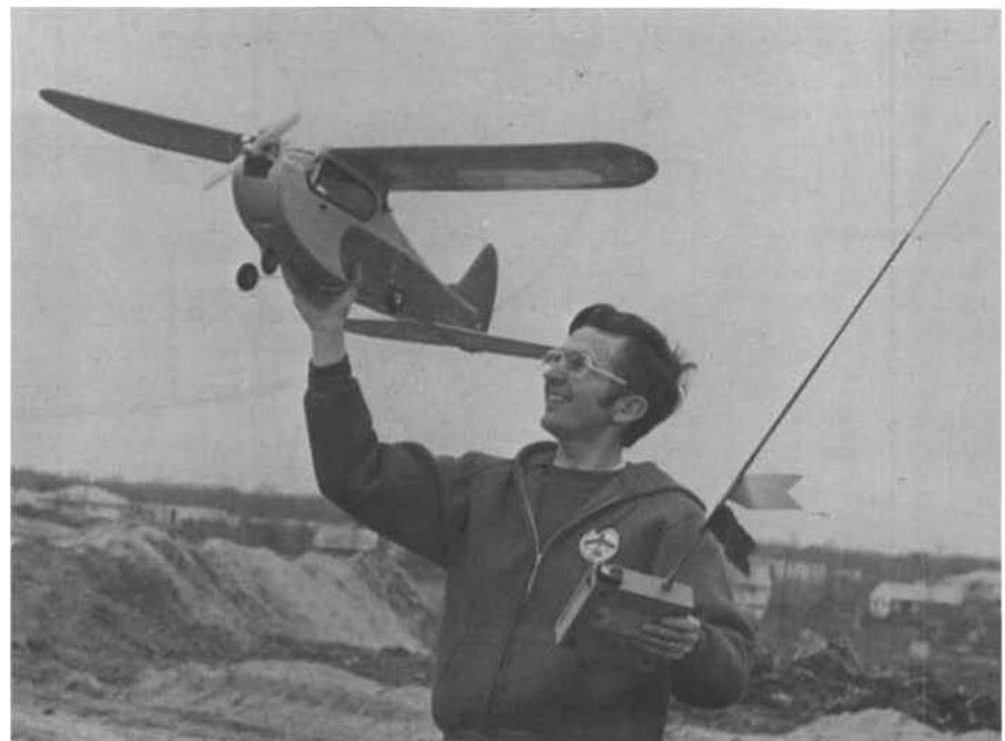
Hand launching, shown by the author, was the accepted method of getting an R/C model into the air. If you had a good throwing arm, you could be the most popular guy at the flying field!
