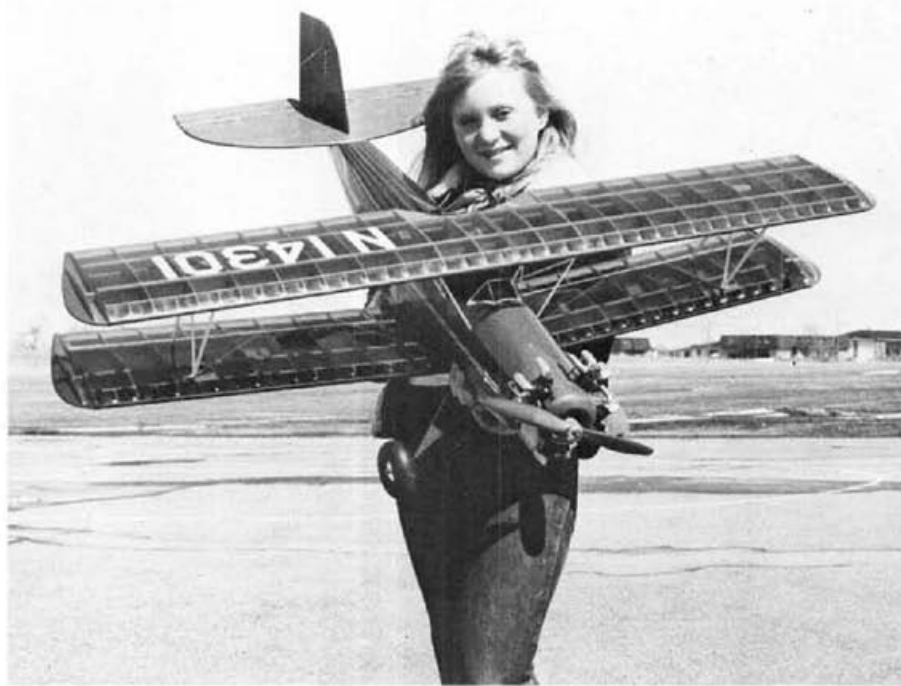
Romey Bukolt's daughter, Susie, holds the Fleet for a size comparison photo. At two inch scale, the span comes out to 49 inches. Performance is brisk with a 40 engine.
