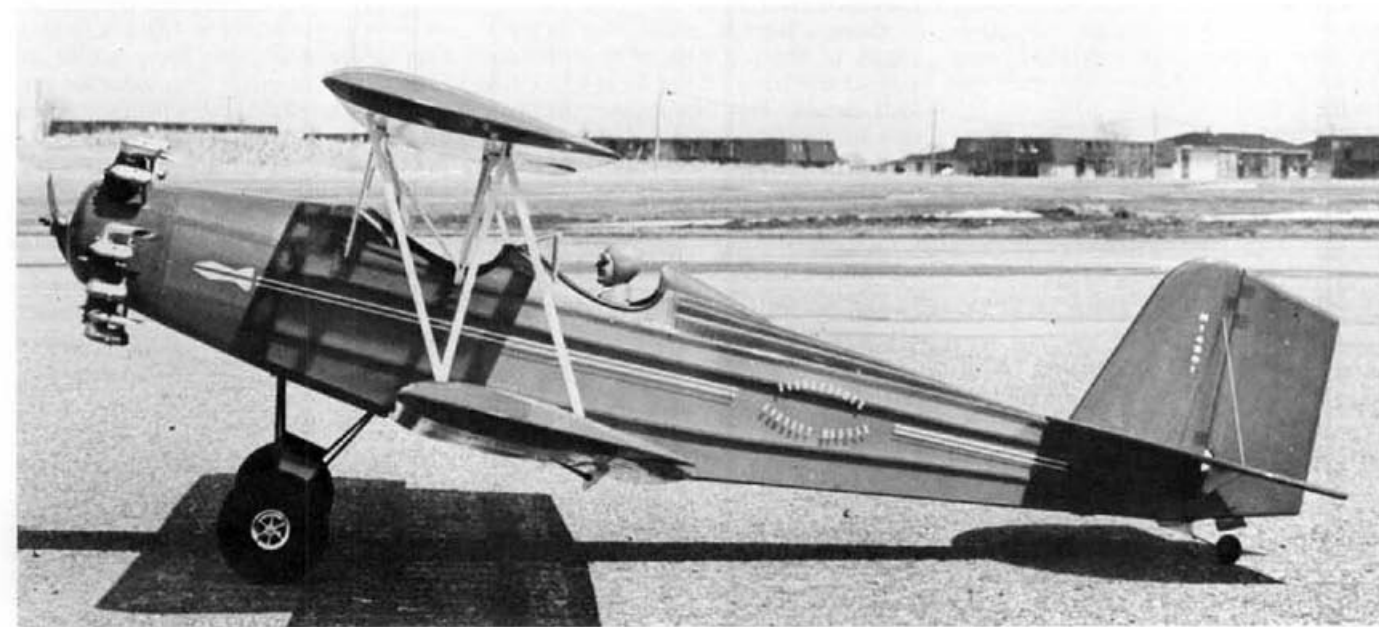
Williams Brothers scale cylinders and pilot add a lot to the realistic appearance of the ship, both on the ground and in the air. Sig Lite-Ply fuselage sides are light in weight, but very strong. Note shadows from side stringers. A kit is about to be released on this model, put out by the author.
