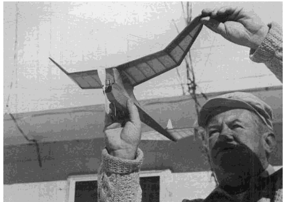
"Ed Toner holding Banshee". This 40% reduction of Leon Shulman's famous design is powered by a Telco Turbotank 3000 CO 2 engine.
