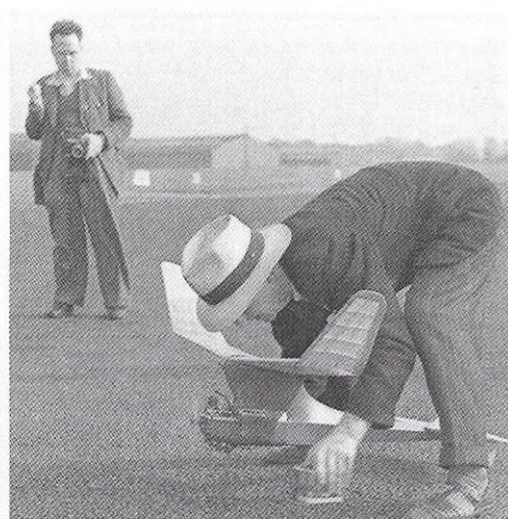
Norman Lees won the petrol competition in the Northern Area Daily Dispatch Rally at Woodford in 1947. Although his model retains the mono-wheel undercarriage and sub-rudders he has fitted an extra spar in the wing and dispensed with the upper leading edge sheeting.
