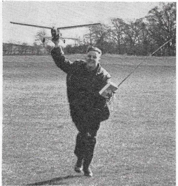
Designer Chris Grubb about to launch "Banker" at the local flying field. This model's smooth, banking turns are a delight to behold, and—once the knack of aileron-flying is acquired—manœuverability is probably more precise than with a yaw-turn type rudder control action.
