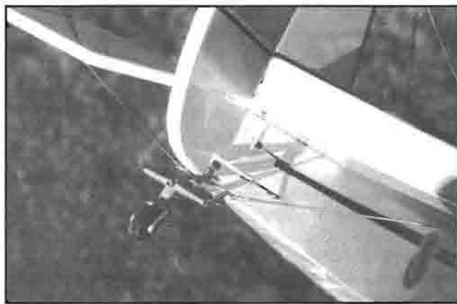
LEFT: Tail braces are 2-56 pushrods with solder links and clevis on ends. Brackets are large Sig landing gear straps. RIGHT: Tail wheel bracket and horn installation.
