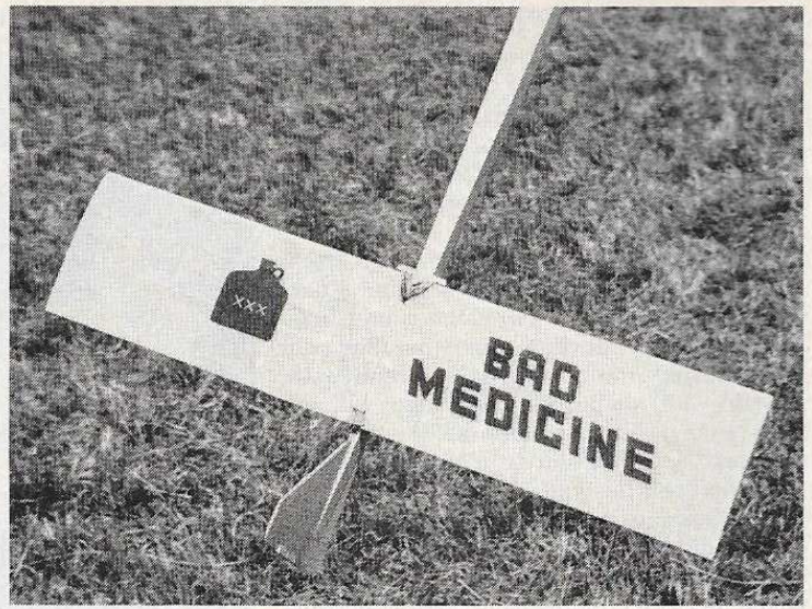
A tale of "Bad Medicine." Fin stays in trim when the stab D-T's upward. Left: Stab pops to angle shown, limited by the line, standard practice. Below: Who dropped what through the wing? Season coming, build it fast!
