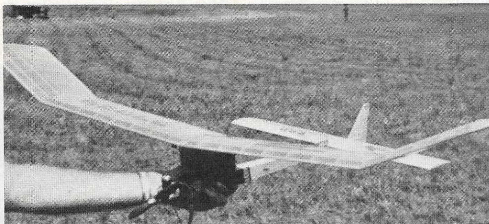
The grass is itchy, it departs earth at great rate. A well tested concept. Design VTO's nicely. Beneath: Coyote food. Kind of typical, but the right amounts of everything to go. Drink up little engine; pressure bladder to force feed its veins. Tatone timer on fuel line, skid saves prop.
