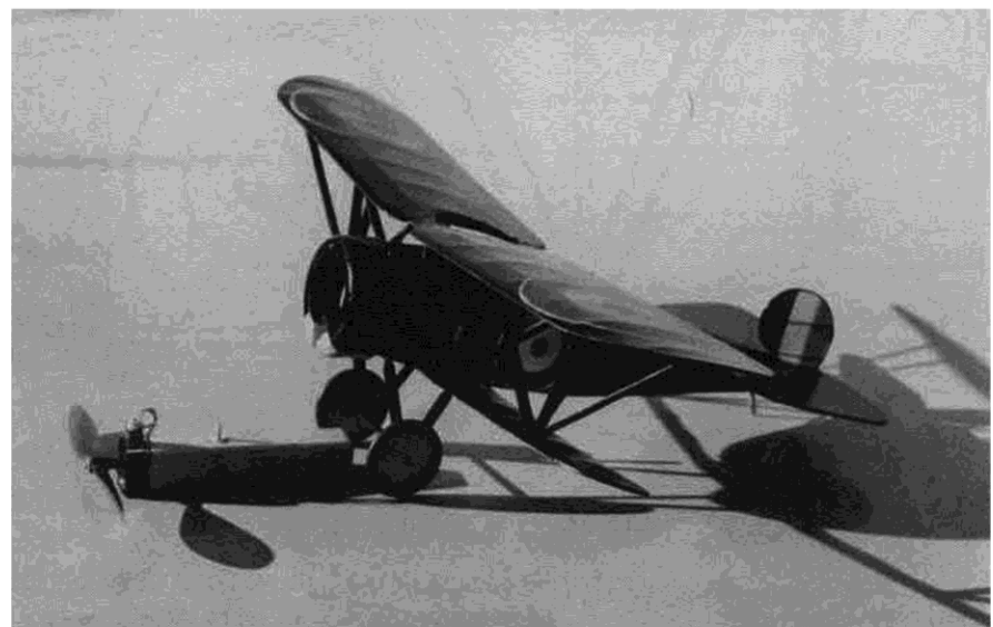
The Spider with its CO 2 unit removed for display. Note the placement of the filler tube.
