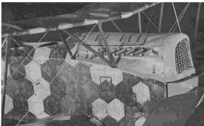
A little bit of engine detailing can go a long way toward adding realism to any model. Aluminum tube exhaust stacks.
