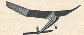
1/2 A BLAZER —Die-cut balsa, tissue, 40" span, for .049 engine. $2.50
