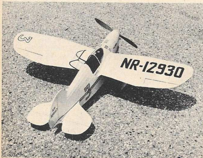
The Jeep was famous for buzzard shaped wings and sleek clean lines. Engine cowling designed for minimum frontal area, max. cooling.
