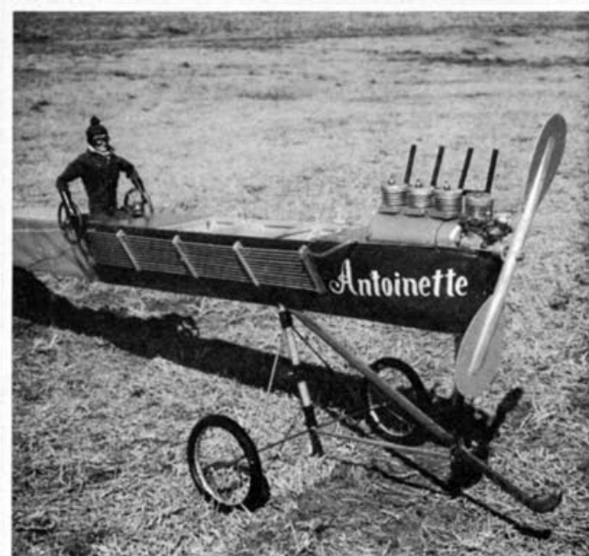
Intrepid aviator views one real, three fake cylinders (hiding fuel tank), and a real Fox 36RC. Landing gear prevents nose-overs.
