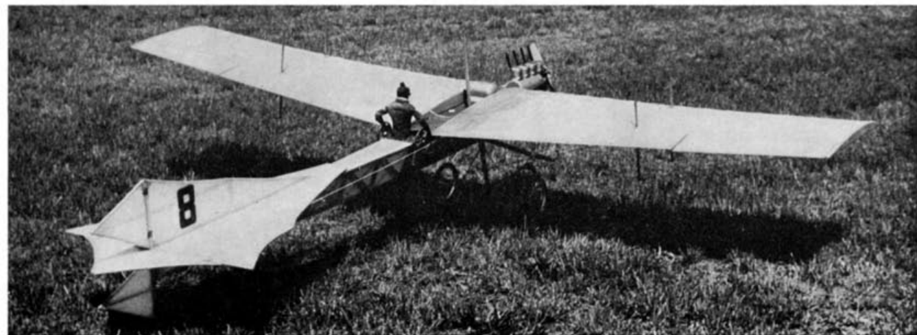
Takeoff must be directly into the wind. Acceleration is slow. Large stabilizer helps with excellent pitch stability and control.
