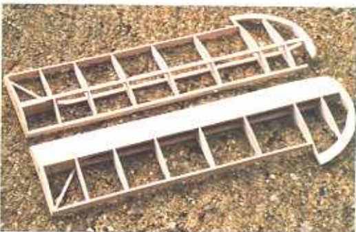
The traditionally built outer wing panels utilise brass joiners.
