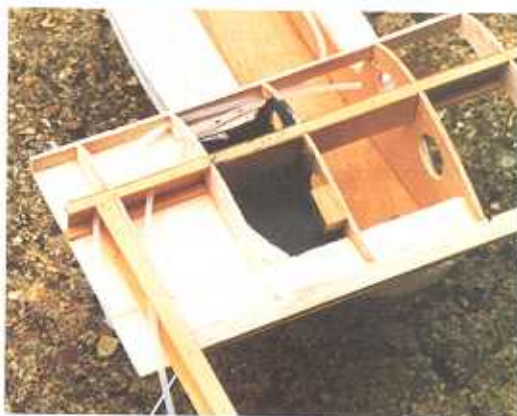
A close up of the wings center panel, note the use of Cyparis for the spars and the booms.
