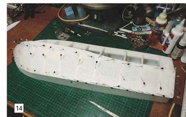
BELOW: Once happy with the side skins trimmed and sanded to size, coat the relevant edges with glue, position and pin on the first bottom skin, and allow to dry.
