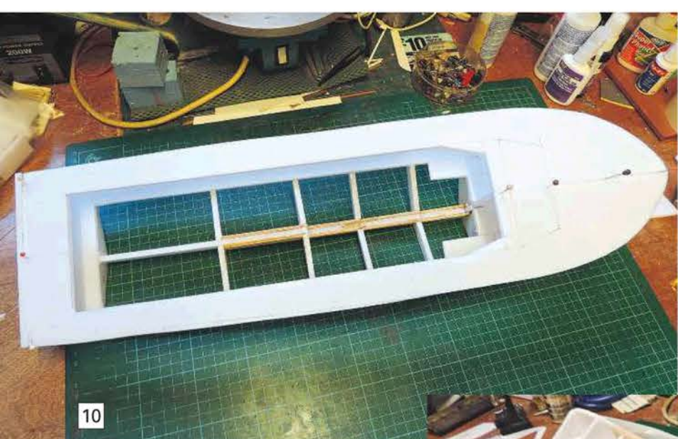
ABOVE: Pin and glue the top deck into the recess in the transom piece and ensuring it is central, the forward part to the front deck support.
