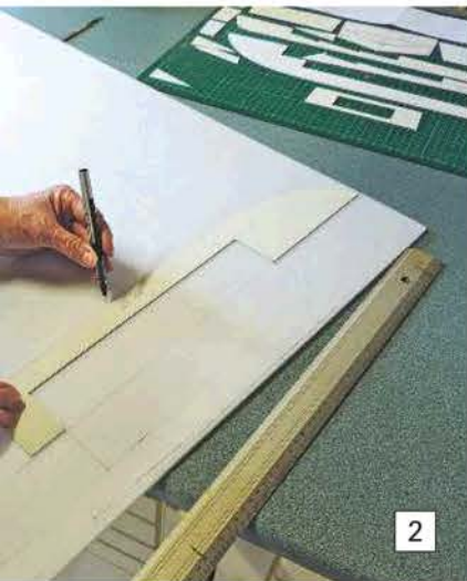
ABOVE: This photo shows the decking piece being drawn so that you have a one piece deck. Check that the complete piece will clear the edge of the sheet of Depron when flipped over, then draw a centre line.
