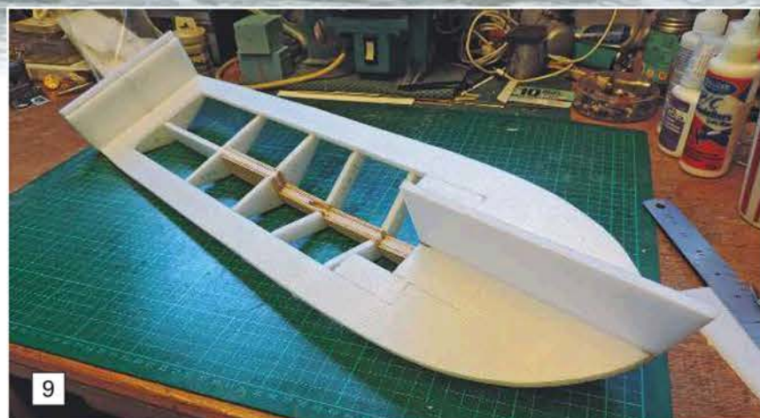
ABOVE: Glue the transom assembly and the front deck support on the centre line. Ensure they are at 90 degrees, although the side formers, if they are cut accurately, will ensure the correct angles.
