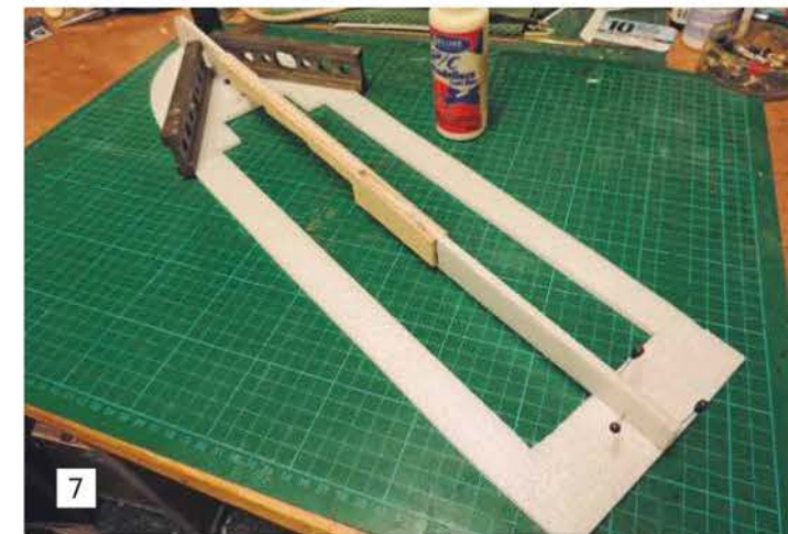
BELOW: Using pins and some 90 degree weights, glue the assembled keel on the centre line of the chine deck and leave to dry.
