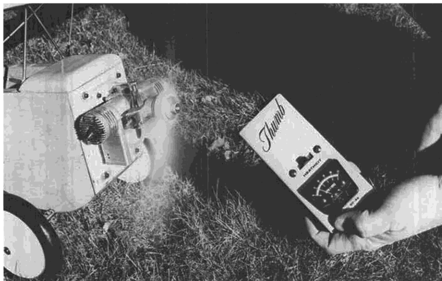
Proof positive! Lengthened venturi and exhaust restricted to those two small holes, gives 5K on 10% nitro fuel and 12 x 6 Top Flite Power Prop. Also very quiet. Photo by Emil Neely.
