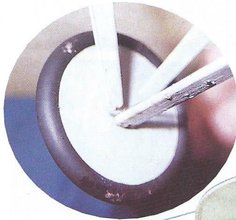
BELOW LEFT: view of the fuselage pod underside, showing the undercarriage struts, receiver installation and the dummy control runs. BELOW: detail of the mail wheel and undercarriage struts.
