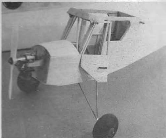
Engine is fitted to firewall. Prototype had an old O.S. 30 and it performed great.
