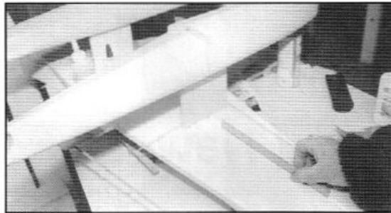
LEFT: Here, 1/8" lite ply is being attached to float keel prior to attaching other side with Tite-Bond glue. RIGHT: Lower spar cap slot is being cleaned out with 1/4" wide sanding bar prior to sliding cap through float pylon and securing.
