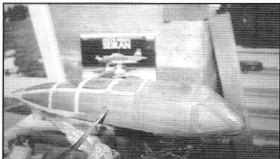
LEFT: After canopy frame was formed with two layers of 3 oz. glass over waxed plug, windows were cut out and frame painted. Windows were glued in last. RIGHT: Cutting foam blocks to shape for floats.
