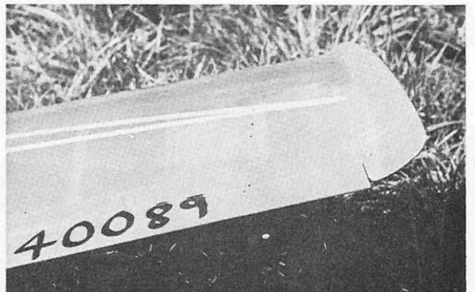
Top left: servo operated 'No load' on-off switch for flight motor. Above right: moulded plastic servo mount used on the original for wing mounted aileron servo. Left: front hatch and wing removed to reveal closely fitting airborne systems. Below: Hoerner anti-vortex tips are employed which contribute to drag reduction.
