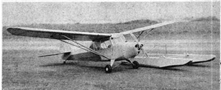
Floats and land gear are quickly interchangeable. Floats are not scale, but are semi-scale and are the proper size. They do work!
