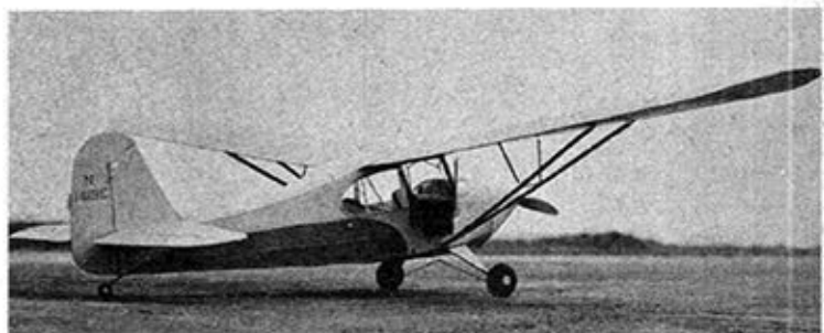
Don't forget to fasten the safety belt. Increased dihedral, slightly enlarged horizontal tail are the only departures from scale.
