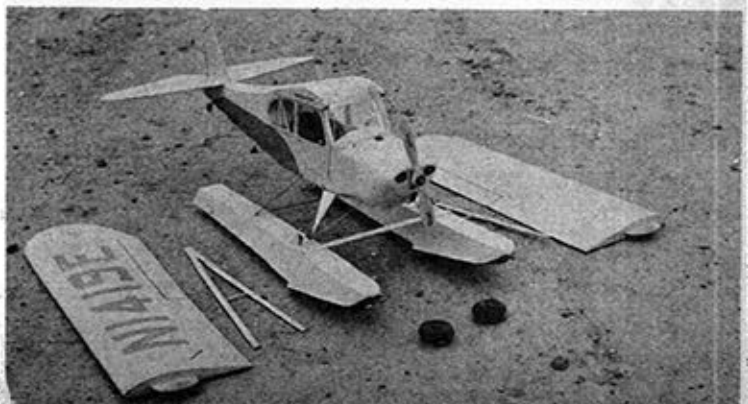
Wing panels knock-off—tongues slide into center-section boxes. Rubber bands looped over wheel hubs give quick float attachment.
