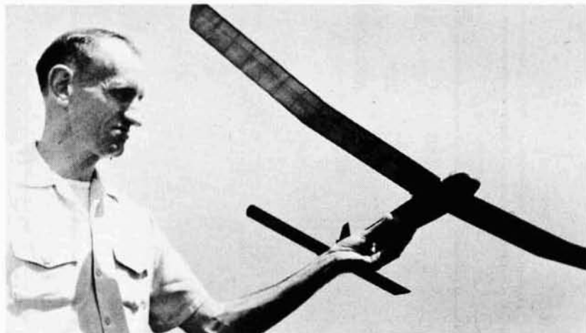
This small handful is an ideal way to get started flying towline gliders. The autorudder and stable design layout make "Aerogull" an easy ship to flight adjust and tow.
