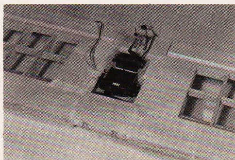
Wing houses aileron and flap servos.
