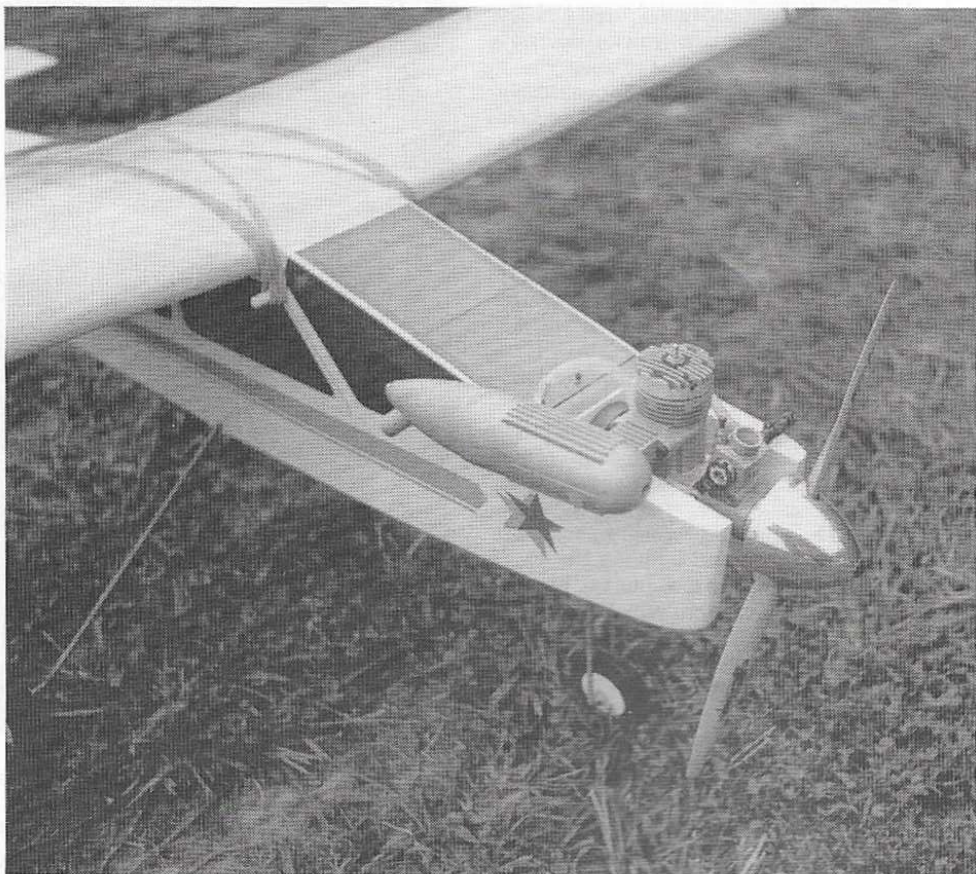
Easily tucked in the nose, the World Engine's A.S.P. .40 (above) provides plenty of power for the model. Climbing out after another takeoff (bottom), the model has very stable response and "grooves" in flight.
