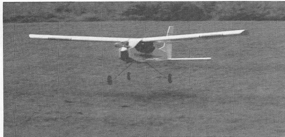
The Aerostar begins to rotate after a short ground run. The wide stance of the \frac{5}{32} music wire landing gear keeps the ground track very straight with no tendency to "squirrel" all over the runway.
