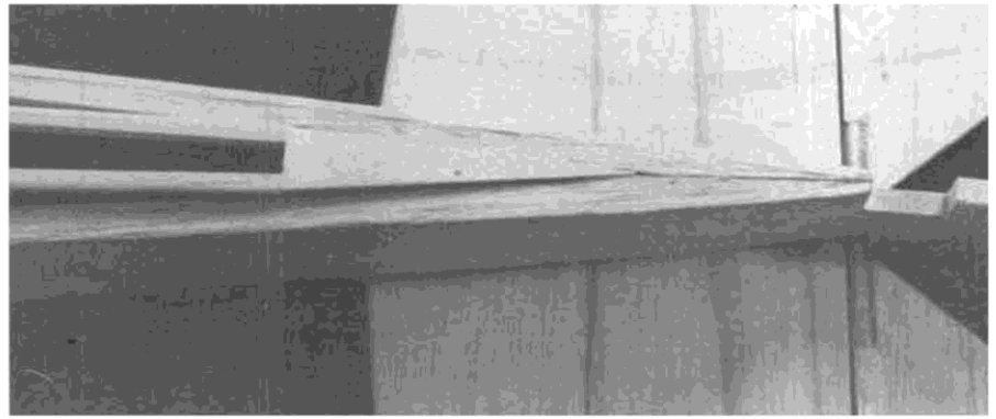
Bottom stringers blend into V-block where sides join at rear. Note hardwood dowel joining elevators, notch in rudder for ply insert.
