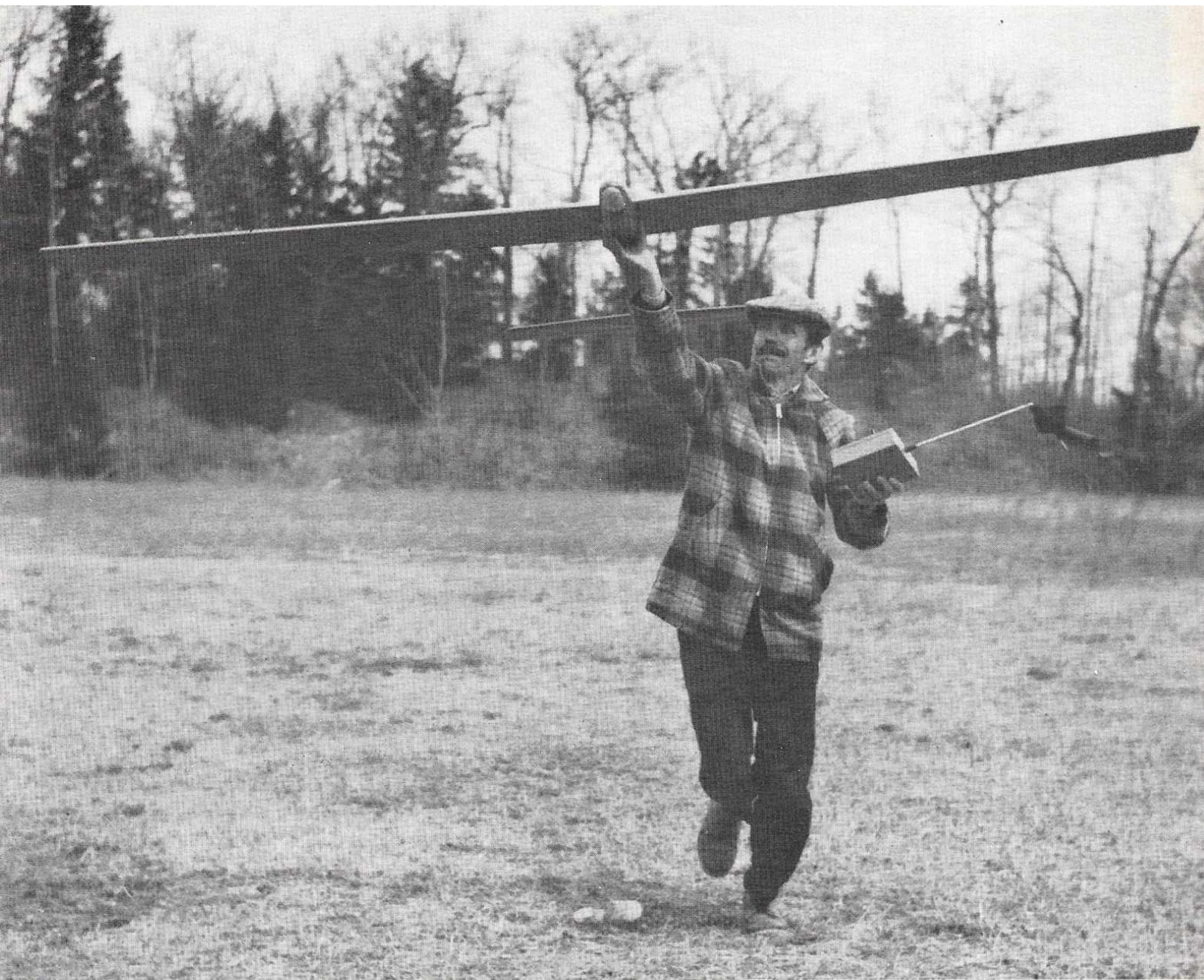
Author demonstrates perfect test glide hand launch; model held high overhead with wing level and transmitter to control direction.
