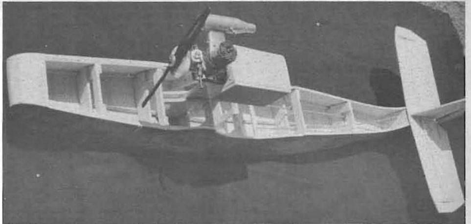
Hull is ready to close up the top. Plans show engine pod tapered at rear for improved looks.
