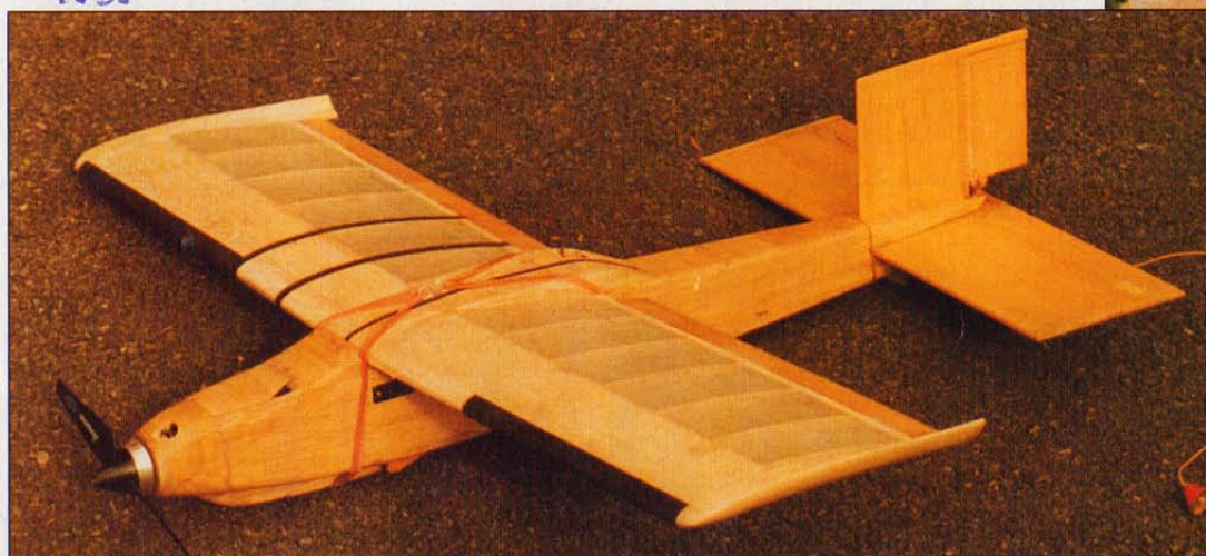
The 384 as it first appeared, powered by the very quiet ED Cadet, 1cc diesel. Its 'transportation box' can be seen behind.
