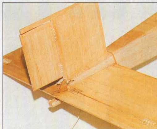
Left: Wing root with wings partly folded to show short locating dowels and 1/64" ply register. One piece wing is a simpler option - 1/16" ply dihedral braces would be necessary though Below: Ply elevator horn with nylon tube bush. Push rod end held in place by spring pressure. Note "stitch" hinges - cheap, simple, reliable.
