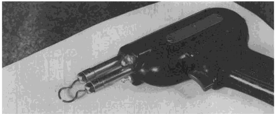
Foam hollowing gadget . . . copper wire loop heated by soldering gun.
