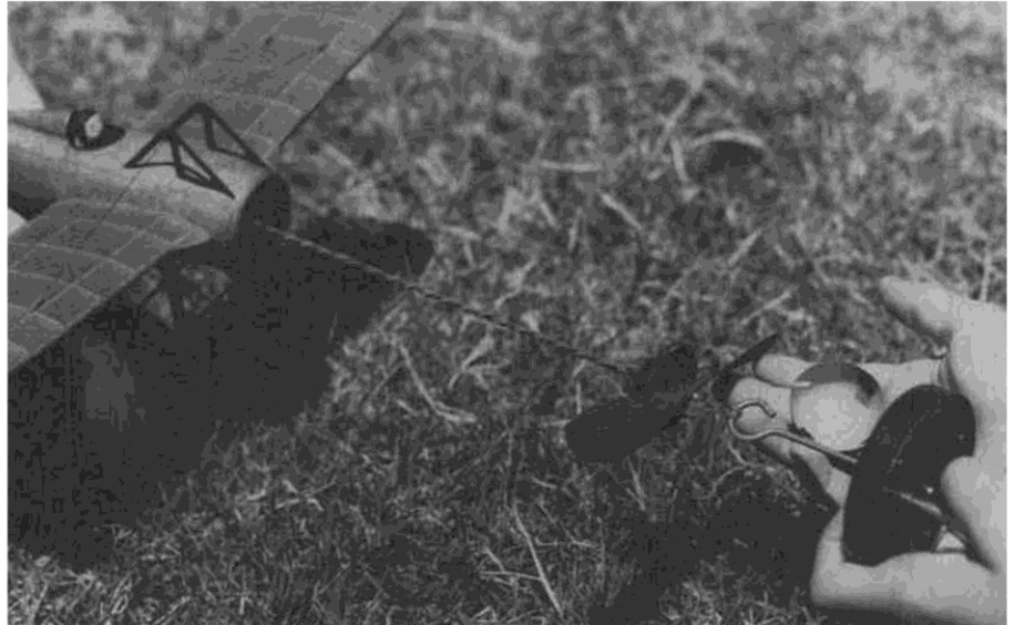
Winding with spinner cap pulled off. Small bits of Velcro hold spinner to back-plate.
