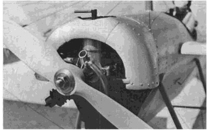
Close-up of engine installation on model, also cowl riveting. Original model used .06 diesel.
