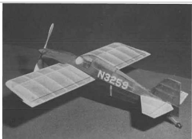
Only deviations from scale are a slight increase in stab area and an 1/8th inch of dihedral added to the otherwise flat wing.
