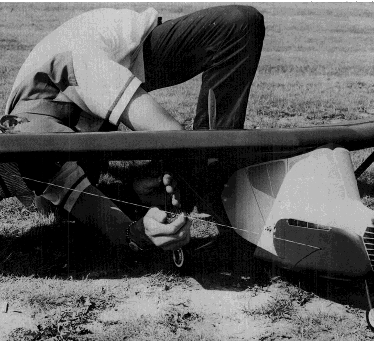
Earl attaches the wing struts before flying the R/C version of Waldo Waterman's Arrowbile.
