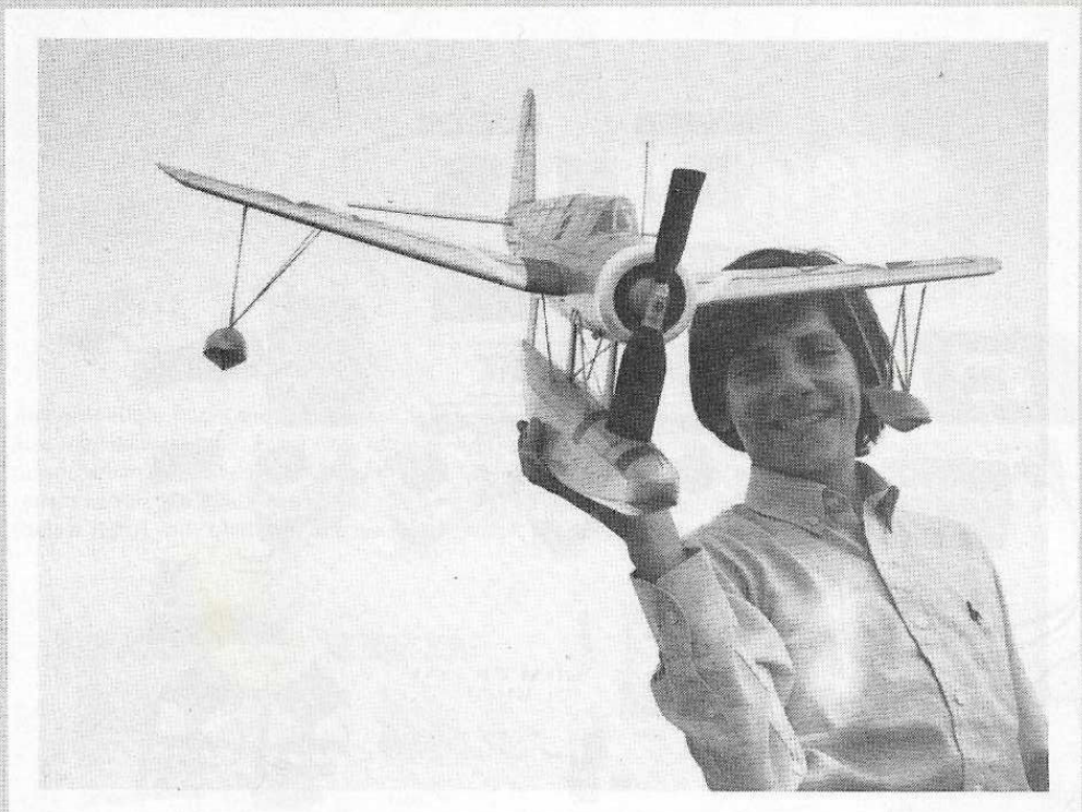
Cory Capps shows off the float version with its eight inch diameter prop (above left); land version uses a ten inch prop. The assembled wing panels show (above right) the plug-in dowels used to attach to the fuselage. The center float attached to the fuselage (below); the float is a built-up structure. Keep it light.
