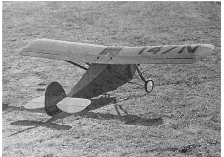
All control surfaces are scale size. Note use of MonoKote strips to simulate divisions of the "window" in the wing over cockpit area.
