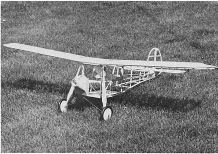
Three-quarter left front view of the Velie Monocoupe uncovered framework.
