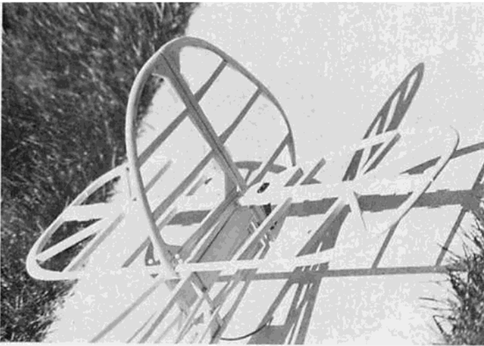
Close-up of uncovered Velie Monocoupe empennage. Light structure keeps weight down in the tail section.
