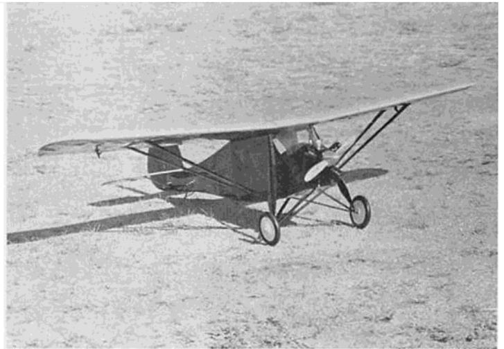
Three-quarter right front view of completed Velie. Strut installation shown. More complex looking than it is to build.
