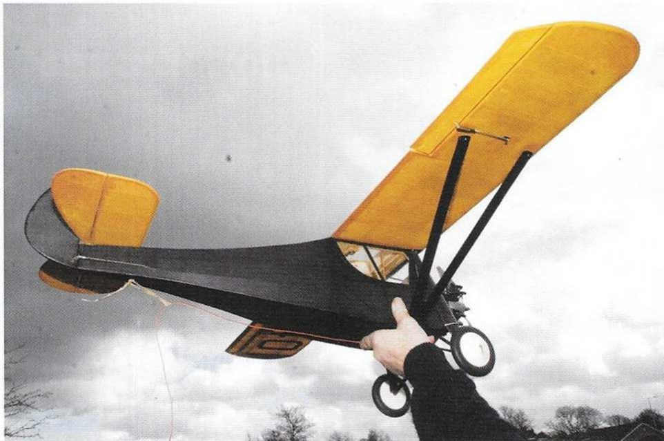
Rear three-quarter view emphasises the short nose moment, so be sure to keep the tail-end light to avoid a balance-point problem.
