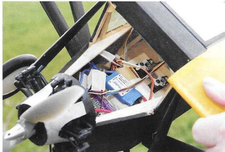
BELOW LEFT: The Cockpit windscreen access hatch - a very neat access arrangement. BELOW RIGHT: Servos, Li-Po battery and motor speed controller under the windscreen hatch.
