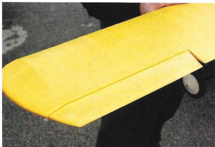
ABOVE LEFT: Countersunk wing retainers bolts at the wing rear centre section. ABOVE RIGHT: Detail of the aileron, that is top surface hinged.
