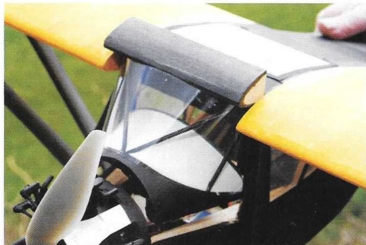
BELOW LEFT: The Cockpit windscreen access hatch - a very neat access arrangement. BELOW RIGHT: Servos, Li-Po battery and motor speed controller under the windscreen hatch.
