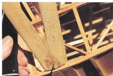
RIGHT: The lower anchor point for the V-shaped wing struts showing the attachment to the fuselage lower side. BELOW LEFT: The finished, covered wing, respendent in yellow tissue, showing the wing strut attachment and the aileron servo link. BELOW RIGHT: Tailskid is a simple piano wire arrangement.
