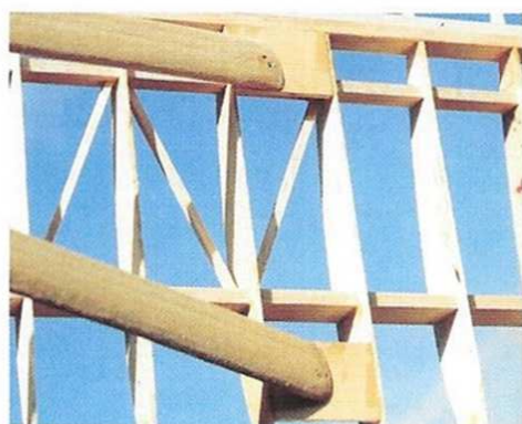
ABOVE LEFT: The completed, uncovered tailplane and elevator, built up over a sheet balsa core outline as per the fin and rudder. ABOVE RIGHT: The finished wing skeleton ready for covering. Phil used tissue to cover this model in preference to the commercially available heat-shrink coverings so widely used these days. RIGHT: Detail of the wing strut anchor points on the underside of the uncovered wing.
