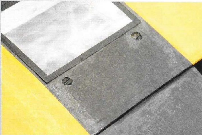
ABOVE LEFT: Countersunk wing retainers bolts at the wing rear centre section. ABOVE RIGHT: Detail of the aileron, that is top surface hinged.
