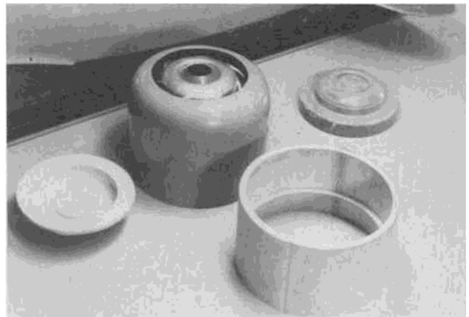
Finished and incomplete cowls . . . all-wood construction. Exhaust collector ring is molded fibreglass.
