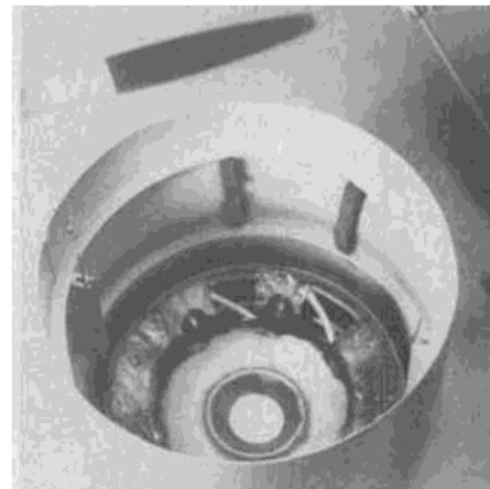
Inside of cowl, showing mounting tracks and two air intake openings.
