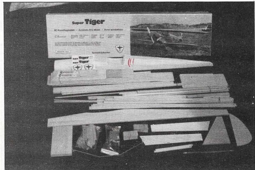
Most identifiable part in the kit spread, below, is the moulded ABS fuselage top decking. Above, basic fuselage components laid out. Note the pre-formed aluminium sheet centre section struts.
