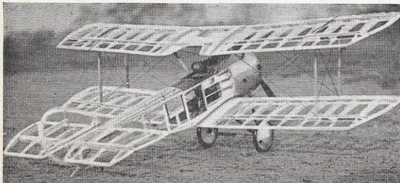
Comparative photographs below, show the McDonough Pup before and after covering. Construction closely follows that on the full size machine as can be seen by study of the 1/72nd scale drawing above. Elevators are specially drooped for realism in the photograph—are pendulum controlled on this 26½ inch span model
