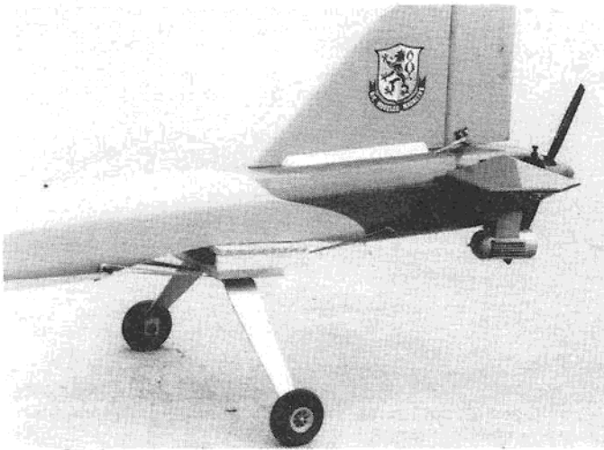
Easy to make rear wheels for transport. Even though the author has never broken the rear stabilator, it is fairly delicate.
