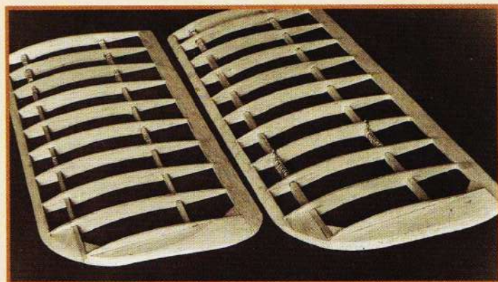
One each of the wing panels, with near-to-scale aerofoil section and thick tips to take care of ground scrapes.
