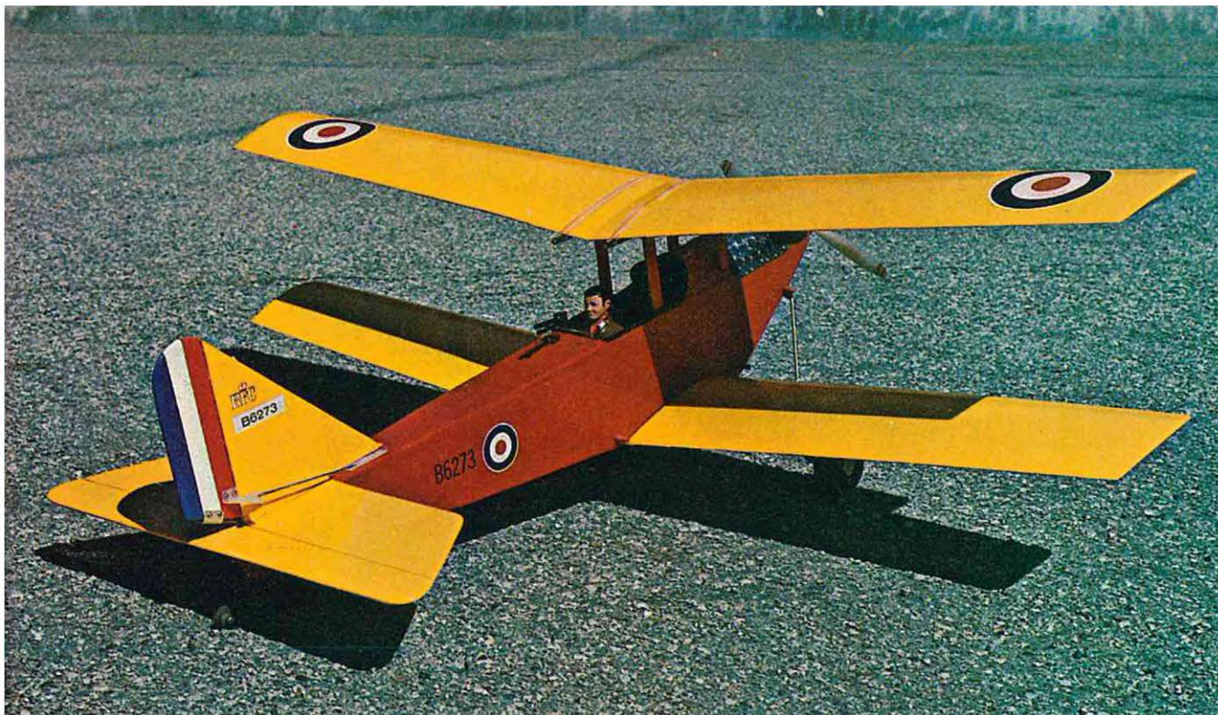
The Rumplestadt after modifications by the British. Transparent orange solarfilm on the fuselage, yellow Solarfilm on foam wings and sheet balsa tail surfaces.
