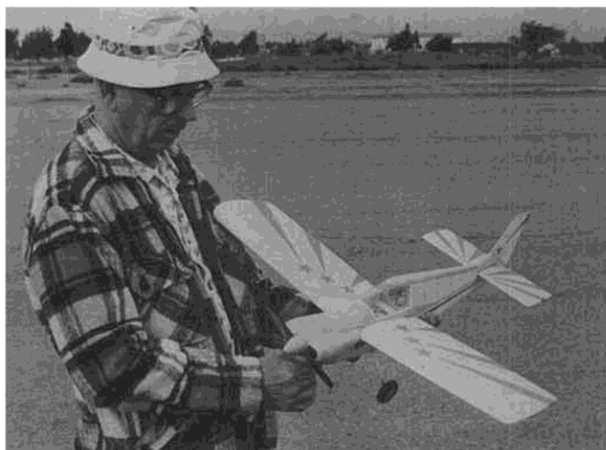
The Pottier is one snazzy looking little airplane, wouldn't you say? Stab mounts with rubber bands, easy to change incidence.
