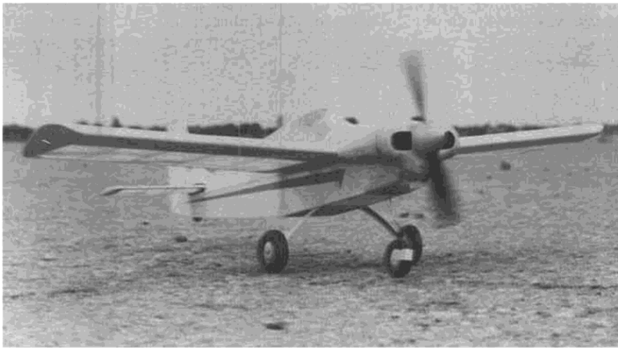
The Pottier just beginning to rotate for takeoff. Nose gear permits straight, stable ground runs, is a real lifesaver when landing in rough areas.
