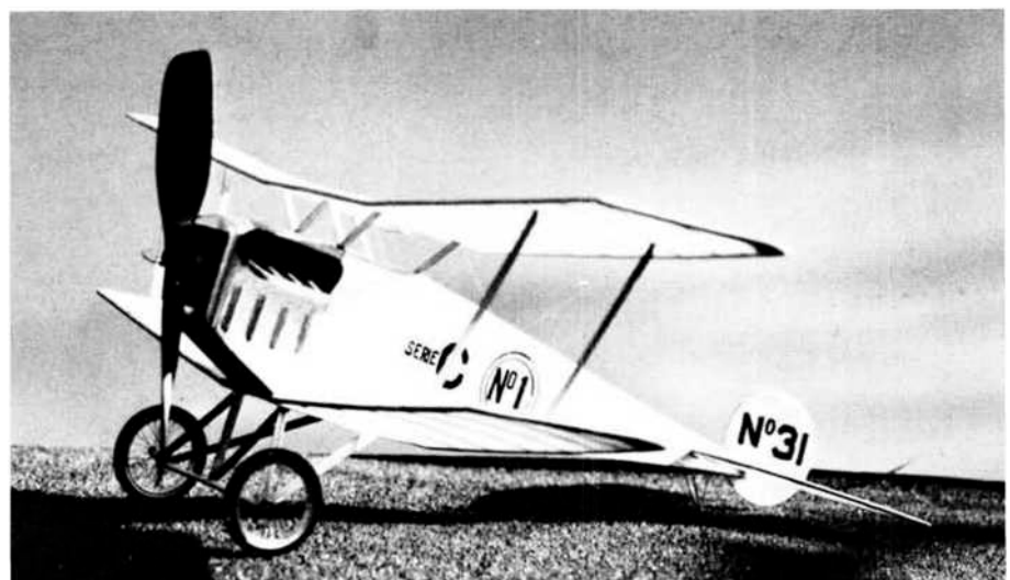
Plane's rather angular lines are sharply contrasted by the circular rudder. Walt found that said rudder had to be increased in size to eliminate Dutch roll. See text.
