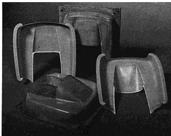
Left: Balsawood and plywood masters from which fiberglass female molds are made from which . . . . Right: Airplane's view of cowling, looking out. Another RCM first (?)
