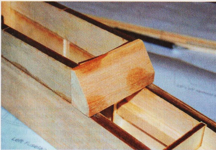
There are many areas of the H-Ray where you can get some easy weight reductions. This solid hard balsa windshield block (above left) can be hollowed. The one-piece main gear was sandwiched between some ply and epoxied into
