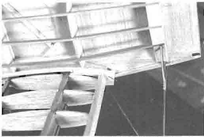
Fitting the lower wing root riblets. Note the 1/32" sheet packing pinned in place.
