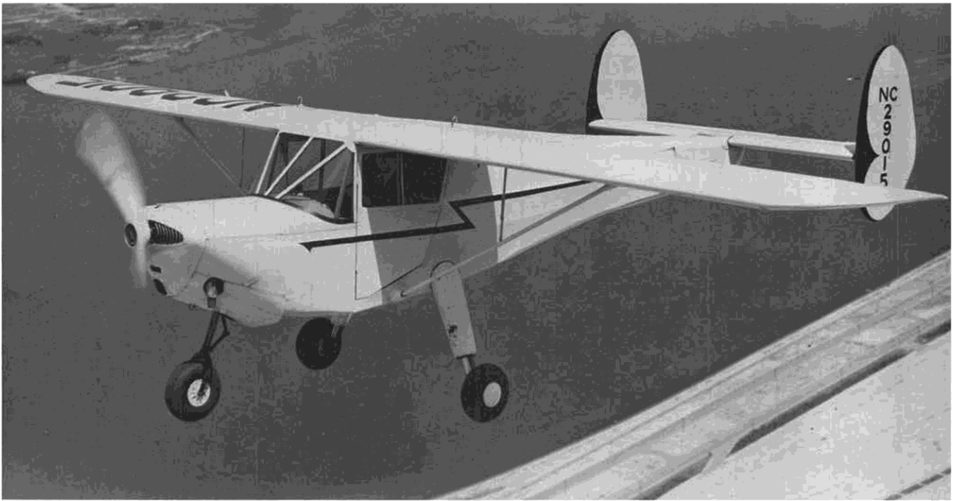
Air-to-air photo of the Skyfarer, taken by famous aviation photographer Rudy Arnold. Fins were fixed, and like the "Erpcup", the plane could not be over-controlled. The opening of World War II put an end to its career.
