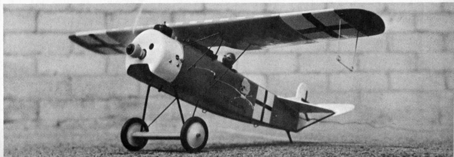
Tied down with engine at full revs makes for an interesting view of the well detailed plane. Note line leadout guides extending beneath the wing.
