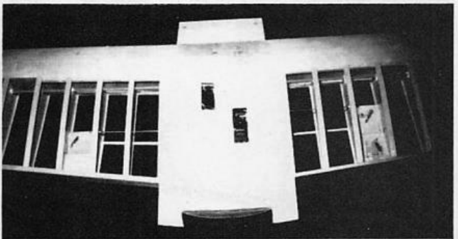
Wing root glassed, servos and links installed, ready for covering. Additional sheet aft of flap bellcranks is optional.
