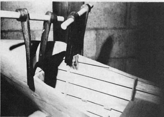
Installing rear wing hold-down blocks. Two more are installed up front.
